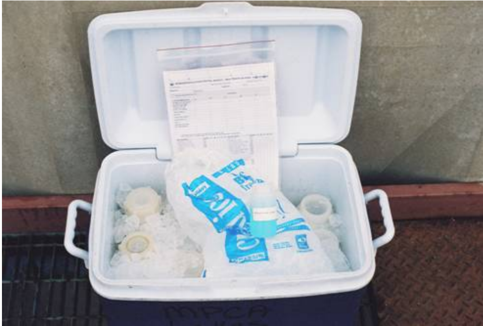
Figure I-1. How to Pack a Cooler. Properly Iced Sample Cooler with a Zip-Loc Bagged Laboratory Sheet and a Shipping Temperature-Check (the blue) Bottle.
