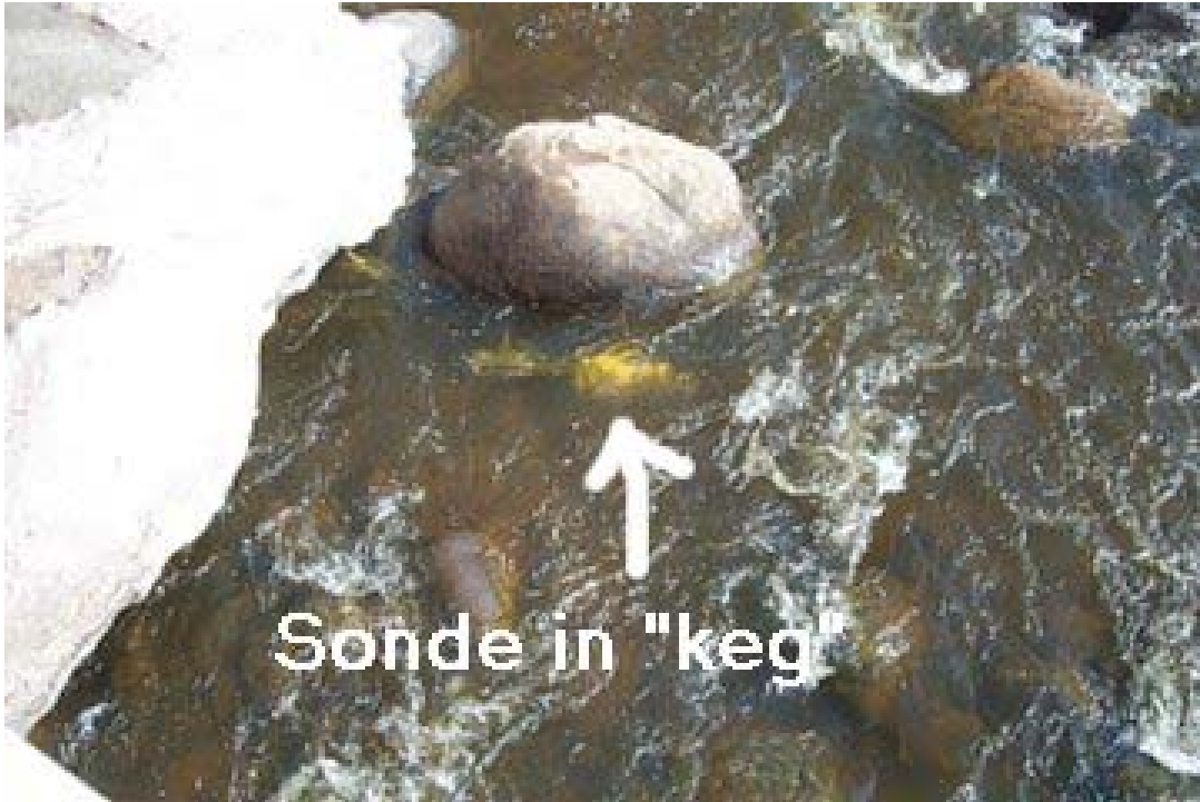
Figure 1. The initial (failed) sonde holder and location. The three cables secured the "keg", one downstream of the big rock, one perpendicular to the current and the third angled upstream.
