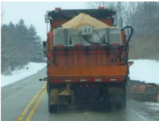
Photo: MCDOT Traveling at slower speeds helps crews use less salt.
