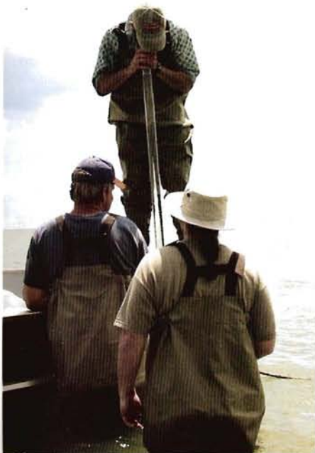
Demonstrating the use of a “transparency tube” for measuring water clarity.
