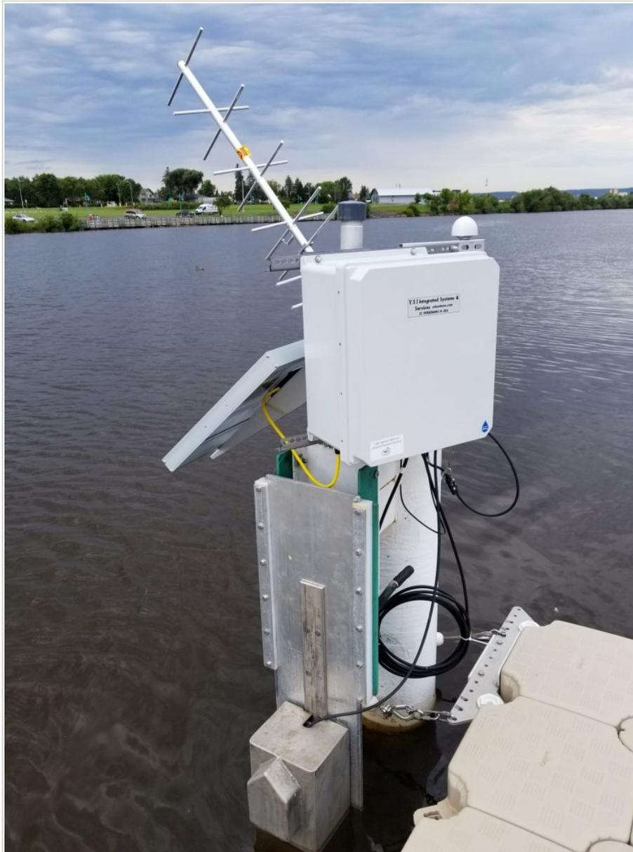
Water quality station on Barker's Island which has the EXO2 sonde, Storm 3 data logger (WaterLog and GOES (Geostationary Operational Environmental Satellite) transmission of data once every hour (Credit: Hannah Ramage)
